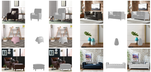
Figure 2. Posed 3D models in catalog images. We use instance masks to automatically generate 6-DOF pose annotations.
